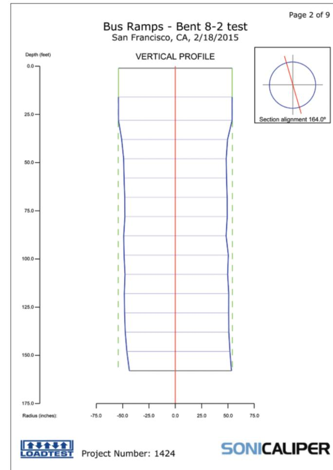
tor the shafts alignment and plumbness. All shafts were accepted and met the project specifications.
