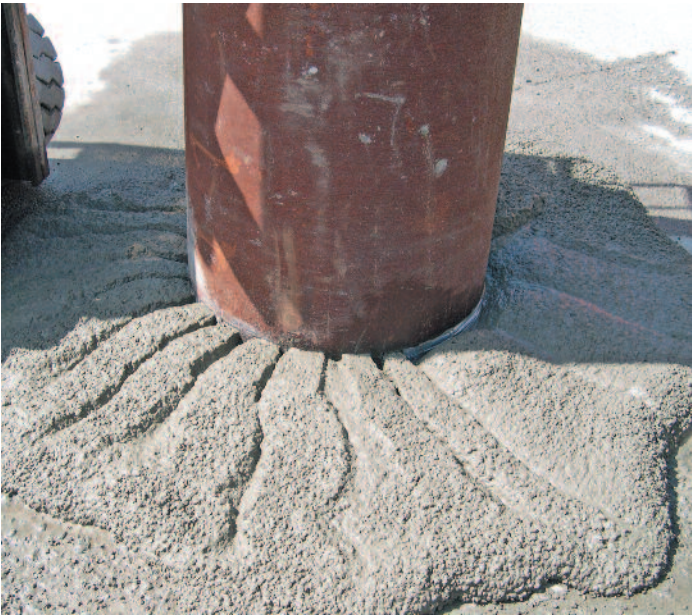
Concrete flowability testing apparatus used to test the mix.
